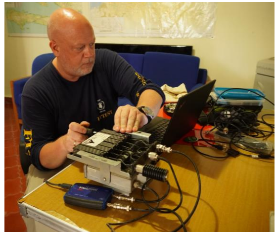
A WFP FITTEST technician prepares VHF repeater equipment for installation in Jeremie, south western Haiti.
