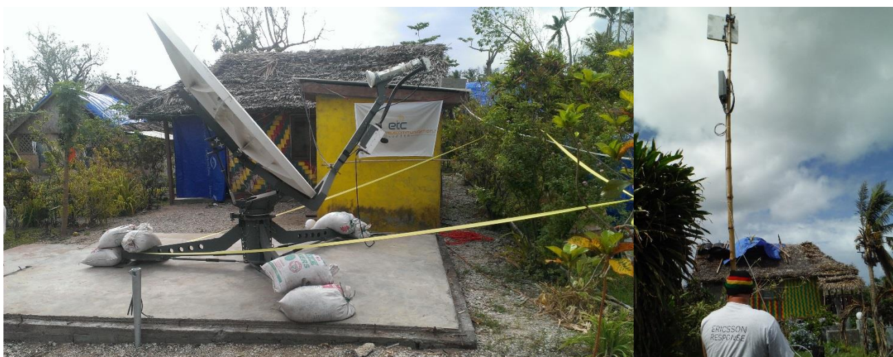
Emergency.lu VSAT & Ericsson Response WIDER equipment set-up at the Samaritan's Purse office on Tanna Island to support the humanitarian community. Photo: Ericsson Response/ Mike Duffin; Ericsson Response/ Daniel Schott
