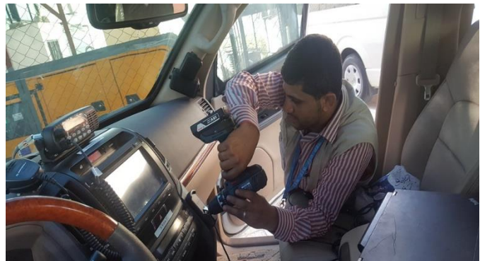
The ETC installing communications equipment in armoured vehicles for IOM in Aden.
