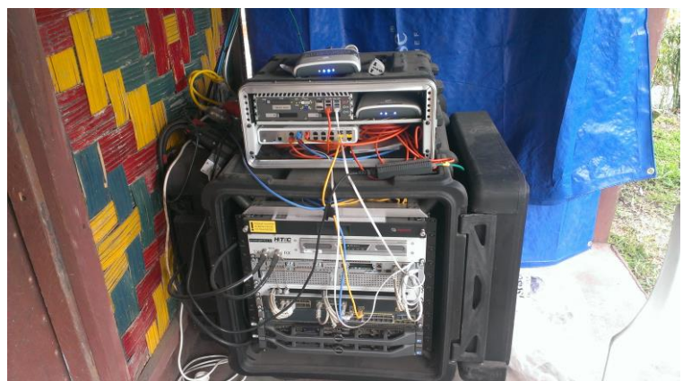
Ericsson Response WIDER and emergency.lu satellite kit continue to provide connectivity at the Samaritan's Purse office on Tanna. Photo: Ericsson Response/ Michael Duffin
